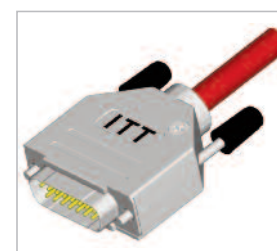
Assemble the other half (screwing force: 100-120 Ncm)
