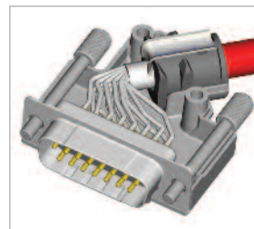
Mount connector and cable into the backshell
