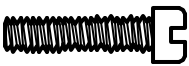
#4-40 x 7/6", fillister head machine screw, C1018 Steel, Zinc Plated (Hexavalent Chromium Free) (2 pcs)
