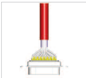
Strip cable 18mm and shape cable to two pigtails
