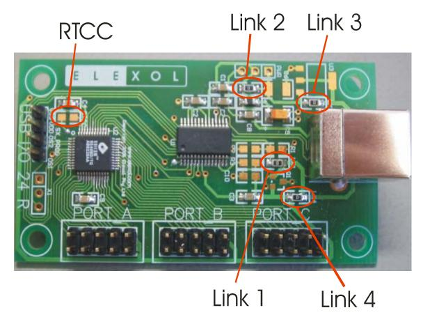
**Link 1** = remove link to use FTDI chip in Self Powered mode. Also remove components C8 and FB. Place components R1, R2. Apply an external power supply (5V MAX) to pin 2 of PWR Connector.
