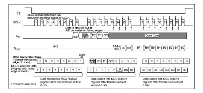
Example image for SPI communications with the MCP3004/3008 using 8 bit segments taken from the MCP3004./3008 datasheet. (http://www.microchip.com)
