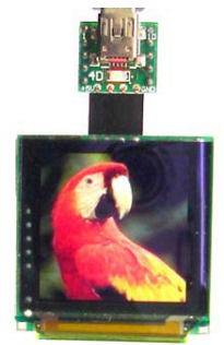
figure 3: Interface to any 4D serial device such as the uLCD-OLED and uVGA modules with the extra 5pin header provided.
