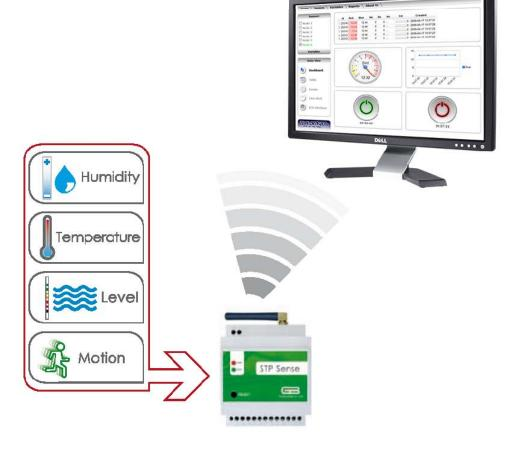
The Smart Terminal SS-STB-B-1 is a powerful remote control and monitoring device. Especially designed for analog sensors monitoring and reporting.
