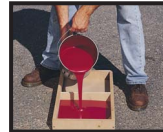
Loctite® Fixmaster® Fast Set Grout Self-leveling, non-shrinking grout for installing machinery and setting anchor bolts. Cures quickly. Can be poured up to 1" thick. Compression strength and chemical resistance are superior to concrete. Forms strong bonds to old concrete and to itself.
