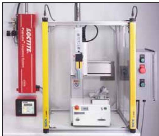
Loctite® Posi-Link™ 10-50 System, Integrated Robotic Solution using a 50 ml dual cartridge, and showing wall-mounted actuator.
