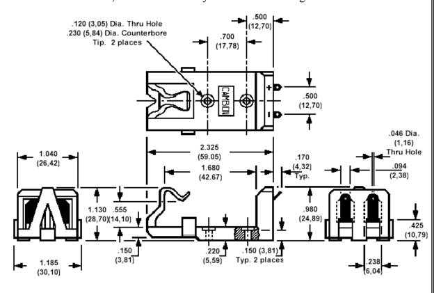
Rec. Mounting Holes - .062 (1,57) Dia., on pitch of 0.500 (12,70) centres, plus bolt down holes per drawing Suited for use on boards up to .125 (3,18) thick
