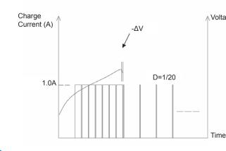
Noltage (V) This charger can charge between 2 and 12 NiMH or NiCd cells connected in series and will detect and provide the correct output voltage and current to suit. End charge is by -∆ V (about 5mV for each cell) detection, after -∆ V. It will turn to trickle-off charge, it's charger current is fast charging current of 1/20.
