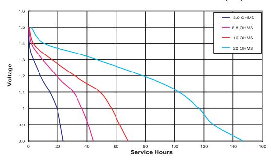
Delivered capacity is dependent on the applied load, operating temperature and cut-off voltage. Please refer to the charts and discharge data shown for examples of the energy / service life that the battery will provide for various load conditions.
