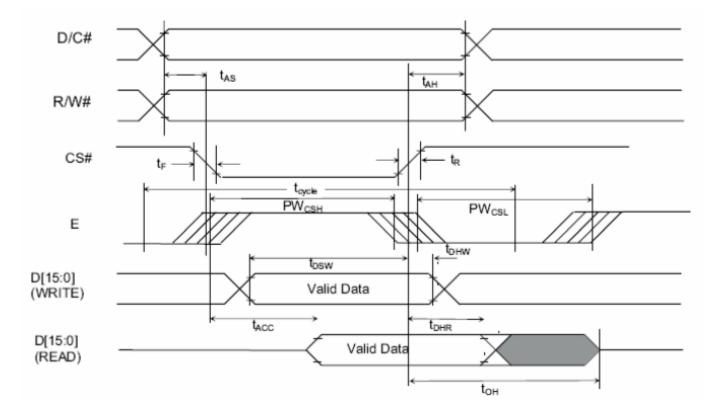
Figure 1 6800-series MPU parallel interface characteristics
