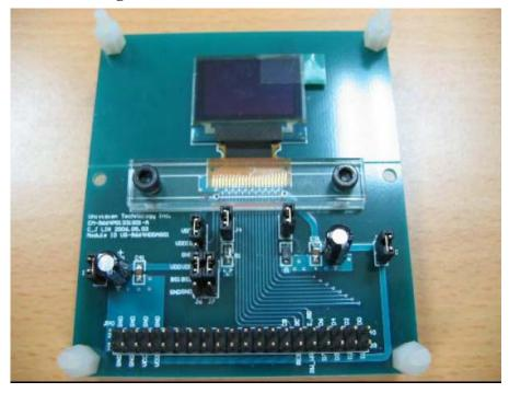
Figure 5 the DD-9664FC-2A and EVK assembled (Top view)
