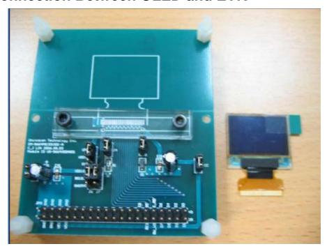
Figure 4 EVK PCB and DD-9664FC-2A Module
