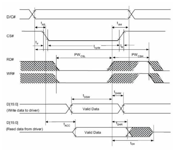
Figure 2 8080-series MPU parallel interface characteristics
