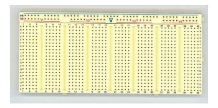
Material: high class POM plastic steel, Dimension: 141.6 x 64.4 x 8.2mm
