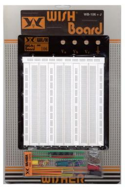
Material: high class ABS plastic, Dimension: 240 x 195 x 31 mm, Distribution strips: 5 Distribution holes: 500, Terminal strips: 3, Terminal holes: 1920,. Aluminium plate thick: 1.5, Knob post: 4, Foot pads: 5 With skin packing
