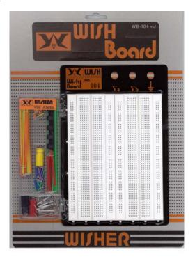
Material: high class ABS plastic, Dimension: 220 x 150 x 31 mm, Distribution strips: 4 Distribution holes: 400, Terminal strips: 2,
