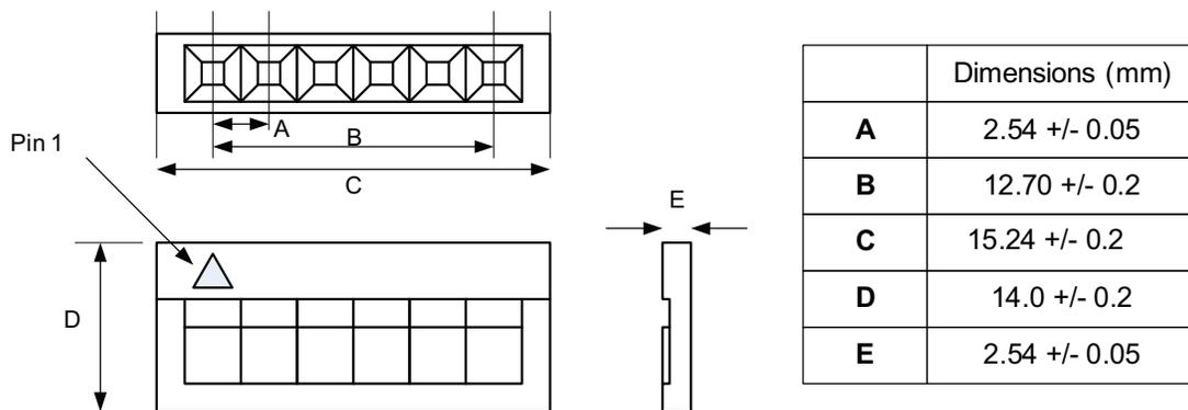
**Figure 4.2 TTL-232R-5V TTL-232R-3V3, 6 Way Header Mechanical Details**
