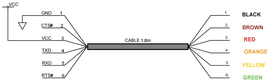
Figure 6.1 TTL-232R-5V-WE and TTL-232R-3V3-WE Connections
