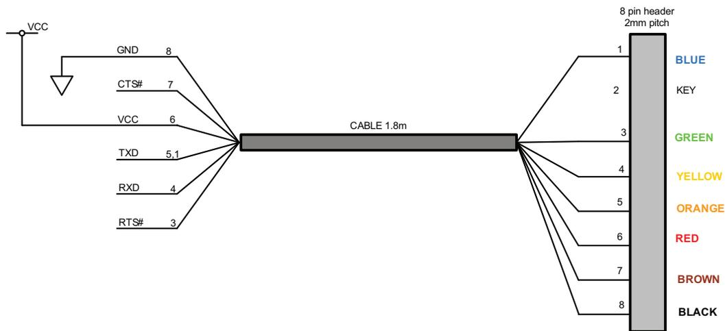
Figure 7.1 TTL-232R-3V3-2mm, 8 Way Header Pin Out
