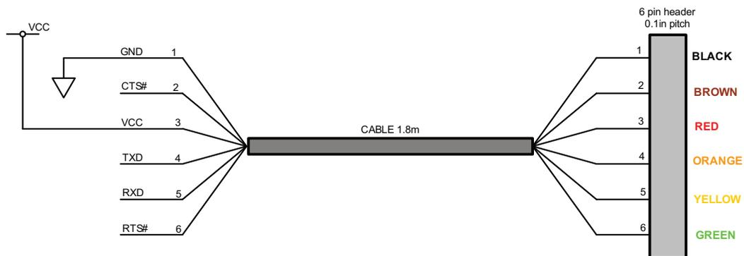
**Figure 4.1 TTL-232R-5V and TTL-232R-3V3, 6 Way Header Pin Out**
