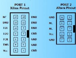
TDI - Data to device TDO - Data from device TCK - Clock signal
