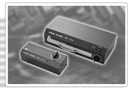
Combine well performance and low cost,LEAP provides EPROM ERASER. LER-121A accommodates 12 devices (24-pin x 0.6"), and suits for small developing environment.
