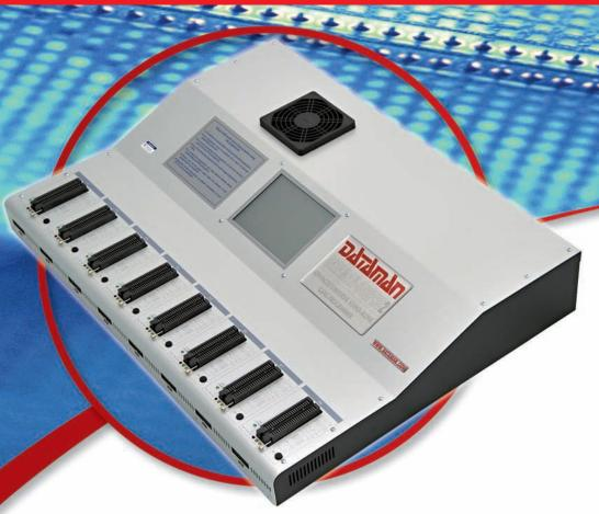
The Dataman 848Pro2 is a super fast stand-alone gang programmer with eight independent 48-pin ZIF sockets, ISP capabilities and internal control PC driven by Windows XP Embedded. The 848Pro2 is built to meet the demands of super fast high volume production programming with minimal operator effort.
