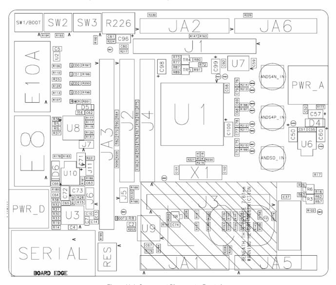
Figure 11-1: Component Placement - Front view
