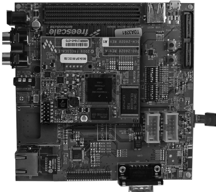
Figure2-7 Connecting the CPU Engine board to Personality board
