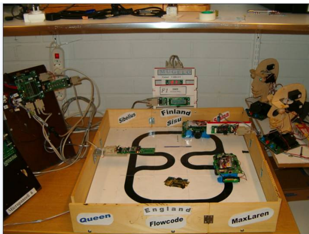
Formula Flowcode with an automatic timing system made with E-blocks and RFID cards.
