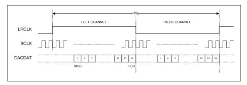
Figure 6 Right Justified Audio Interface (24-bit word length)
