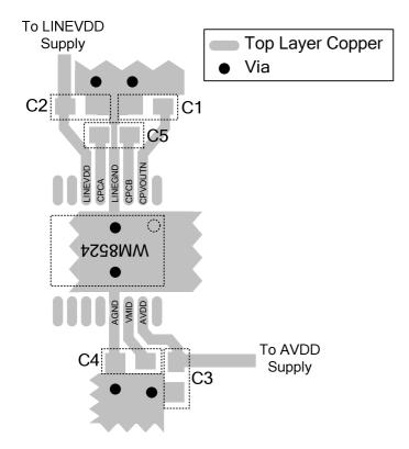
Figure 17 Recommended PCB Layout
