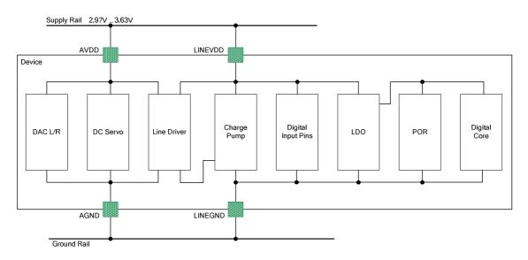
Figure 10 Power Domain Diagram
