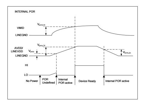
Figure 4 Typical Power Timing Requirements
