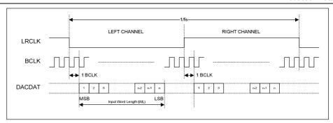
Figure 8 I<sup>2</sup>S Justified Audio Interface (assuming n-bit word length)
