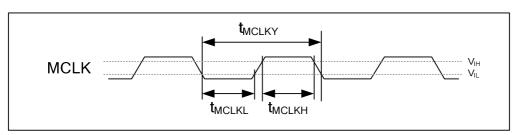
Figure 1 System Clock Timing Requirements
