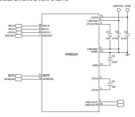
Figure 15 Recommended External Components
