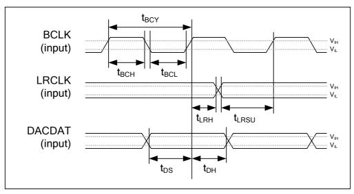
Figure 2 Digital Audio Data Timing - Slave Mode
