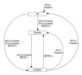
Figure 9 Hardware Power Sequence Diagram
