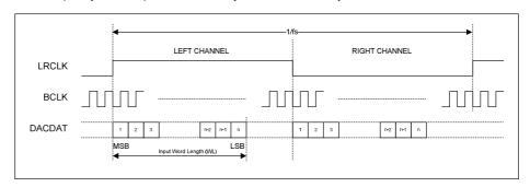
Figure 7 Left Justified Audio Interface (assuming n-bit word length)
