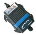
The ARF45 are a family of Serial to Wifi gateways. They permit an immediate connection of any serial device to a Wifi network with an enhanced
