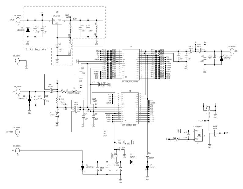
Figure 1. Power Supply, CS5471, and Oscillator
