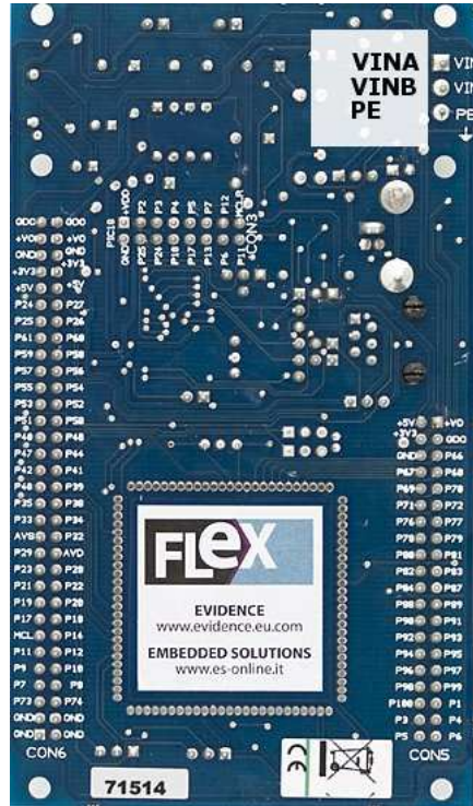
Figure 3.4: Rear view of the FLEX Full version, with highlighted power supply pins (original photo courtesy of Sparkfun).
