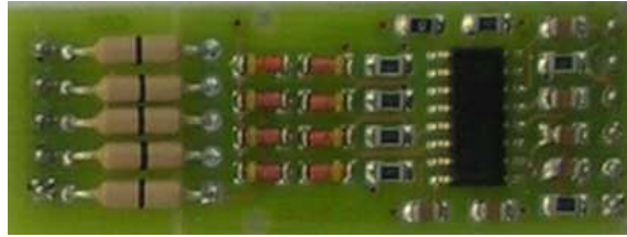
Figure 3.20: The UART TTL module layout.
