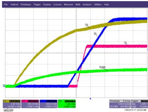
Fig. 7. Start up at 3A Load Ch 1 :V in , Ch 2 :V o , Ch 3 :V SS , Ch 4 :Enable
