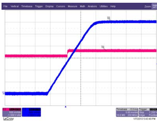
Fig. 9. Start up with 1.62V Pre Bias, 0A Load, Ch 2 :V o , Ch 3 :V SS
