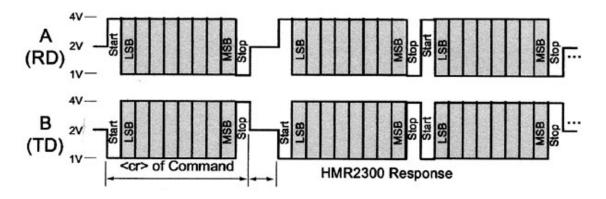
GLOBAL ADDRESS (\*99) DELAY (Timing is Not to Scale)
