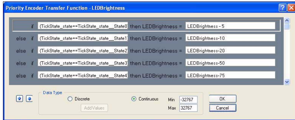
Figure 5-3. Priority Encoder Transfer Function - LEDBrightness
