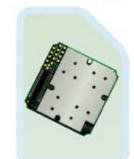
SIM5210 is a HSDPA/WCDMA/GSM/GPRS/EDGE module solution which supports up to 7.2M downlink speed and 384K uplink speed data service. It also has strong capability with rich interfaces including UART, USB2.0, GPIO, TCP/IP protocol stack, etc.
