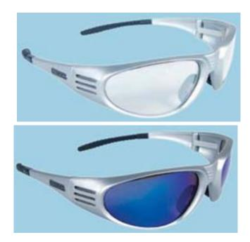
Modern style spectacle with full wraparound frame, soft tipped temples with belt ribs and soft rubber nose piece. Hard coated polycarbonate lense with 99.9% UVA & UVB filter. CE marked to EN 166-1F. Clear or blue lenses.
