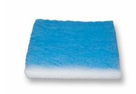
his range of filter media is manufactured as a continuous glass filament to provide a highly-stable air filter medium with an EU3 filtration rating. It has multi-stage filtration characteristics, with an open structure on the upstream face, graduating in density to an integral laminate backing on the downstream side.
