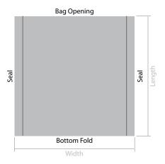
Our bags are manufactured from industry approved polyester and polyethelene laminates. The polyester dielectric works with the metal layer to provide a Faraday effect, the metal layer preventing penetration from damaging electrostatic fields. The specially processed polyethelene keeps tribocharging to a minimum.
