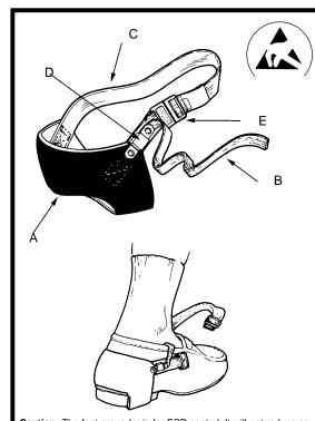
**Caution:** The foot grounder is for ESD control. It will not reduce or increase your risk of receiving electric shock when using or working on electrical equipment.
