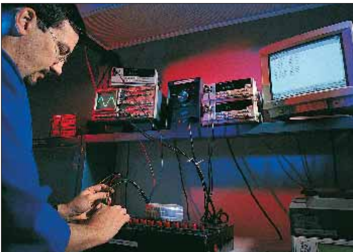
Each AMVECO toroidal transformer is subjected to several tests, including 4kVAC minimum hi-pot testing between primary and secondary windings.
