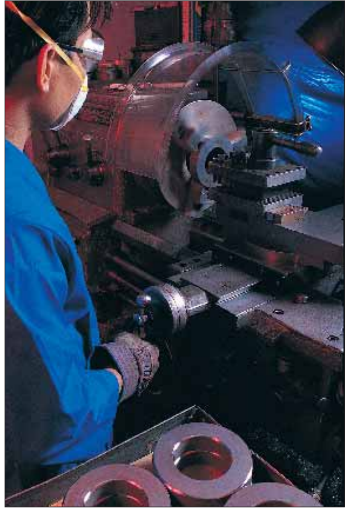
AMVECO toroids are uniquely lathed at the edges of end core to reduce size and increase performance.
