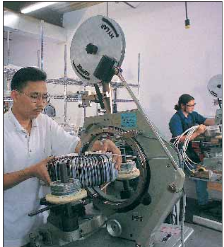
Applying Part of the Insulation System
