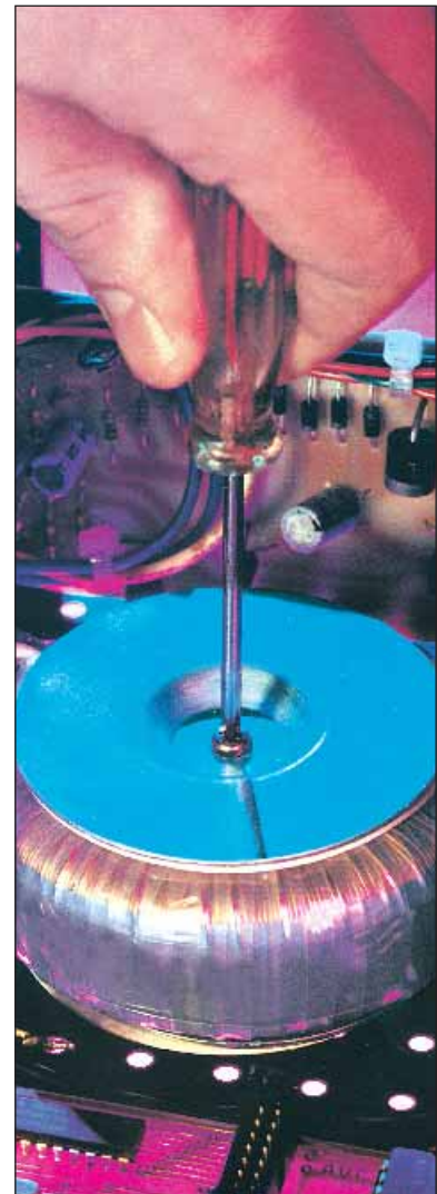
Convenient One-Bolt Mounting
