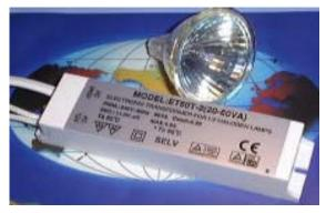
CHARACTERISTICS: Power: 20-60W Terminal blocks or cable connections Input cables (where used): 2x0.75mm2, VDE approved, 23.5cm long Output cables (where used): VDE approved silicon fibre cable, 23.5cm long Input voltage: 220-240V/50Hz (240V nominal for UK) Input current: 0.27A at 60W Output voltage: 11.6V~eff Ambient temperature Ta: Max. 50 degrees celsius Case temperature Tc: Max. 85 degrees celsius Tested in accordance with: EN55015, EN61000, EN61046, EN61547
