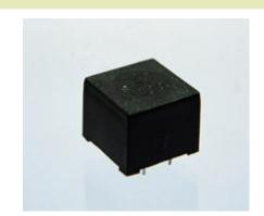
Provides isolation between modems or similar devices and telephone lines. This transformer is designed for use in voice or data transmission circuits where the line d.c. is diverted from the windings by a choke or solid state device. The use of this transformer should enable the equipment it is used with to comply with the relevant requirements of BS6305.
