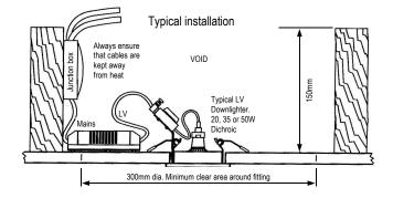
Transformer ratings Primary Voltage (Mains in) 240Volts 50Hz AC Primary running current 0.46 Amps Low Voltage ( Secondary ) 11.6 Volts AC Low Voltage (VA) (Sec) 35-105 VA Max. Sec Amps 8.8 Amps Class III SELV Isolation Class IP Rating
