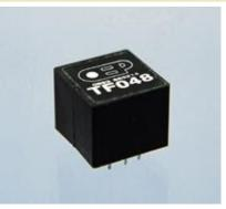
transformer offering improved performance over the OEP1200 and similar devices. A three part concentrically wound bobbin is utilised to provide improved primary to secondary coupling together with improved frequency response and return loss characteristics.
