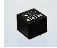
very low distortion version of the industry standard OEP1200 device for use in V.34 applications. In common with that product this transformer is designed for use where the telephone line current is diverted from the winding by a choke or solid state device. Its use will enable users to comply with the requirements of BS6305.
