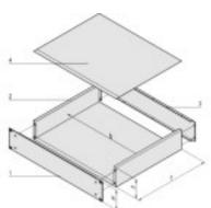
h = clear overall height (H - 3.0), b = clear installation width = 447 mm
