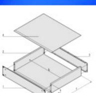
h = clear overall height (H - 3.0), b = clear installation width = 447 mm
