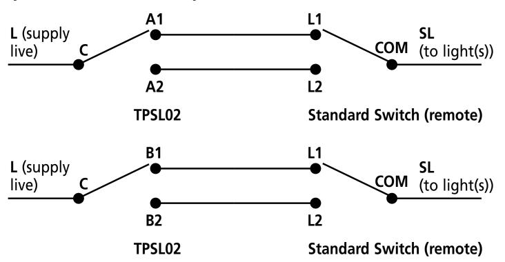
Either standard switch could be a TPSL01 or half a TPSL02). Connections to SL (lights) and L (supply live) can be swapped if required.
