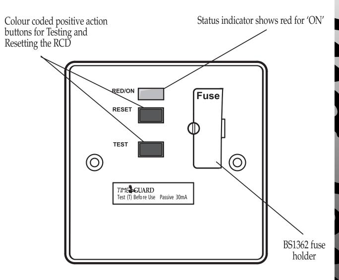
The RCD fused connection unit is a latching (passive) version. If set, this will retain closed contacts if the mains supply is interrupted – essential for applications such as freezers.
