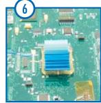
Place the Heat Sink squarely in the Frame Clip over the component. Note the direction of air flow when placing your Heat Sink.
