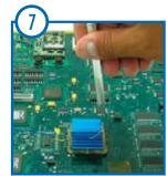
Secure the "Open End" of the Spring Clip under the lip of the frame clip.
