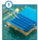
Inspect the installation. Double check to make sure the Heat Sink is securley attached.
