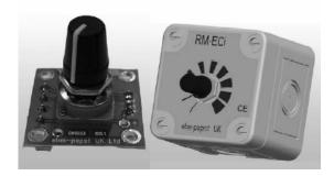
General remarks: ECi controllers are designed for use with the full range of ebm-papst ECi (Electronically Commutated with integrated electronics) fans, they are powered via the DC output from the fan and provide a 0-10V signal to enable infinitely variable speed control. The controllers also enable speed measurement of the fan using a multimeter with a frequency measuring facility ( where a tacho output is provided from the fan).
