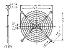
Welded, zinc-plated steel wire
