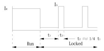
3rd wire signal Run : Square Wave Locked : Vmor VL
