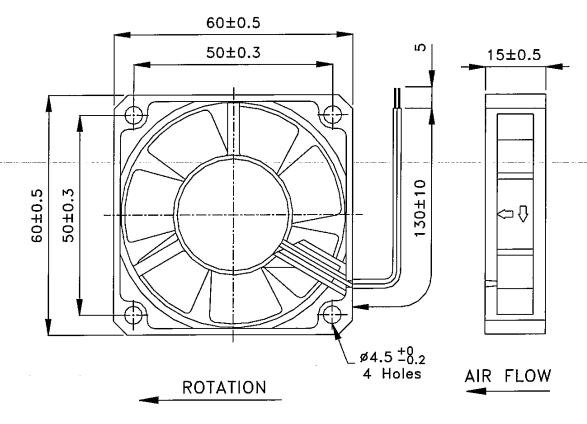
please do not touch and push Fan Blade with fingers or others. Fan Blade and Ball Bearings may be damaged. And it causes noise defect.
