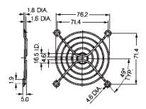
Welded, nickel chrome-plated steel wire
