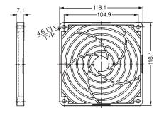
Welded, chrome-plated steel wire.
